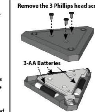
Remove the three Phillips head screws with a 4mm screw driver.
