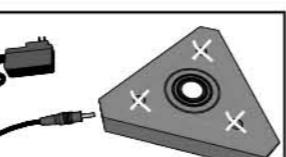
When using an AC Adapter, NEVER place the adapter plug into the Triangle Power Base top peg holes.
