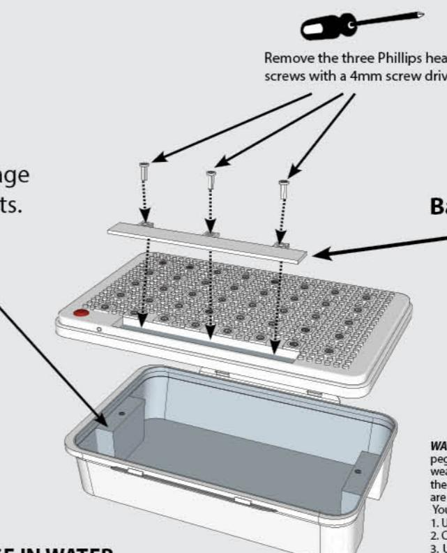
Remove the three Phillips head screws with a 4mm screw driver.
