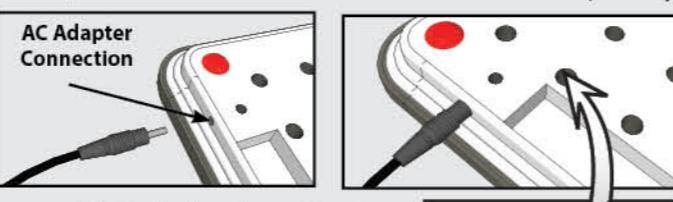
Remove all batteries from Laser Pegs® 3D Lite Board® power base before using 5-volt AC adapter.
